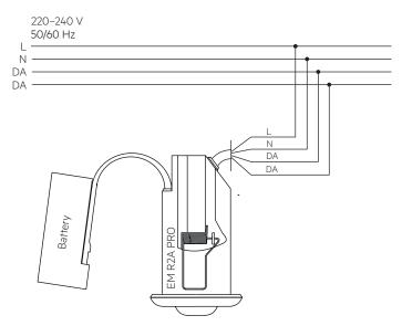
Note: Battery must be connected before mains connection.
