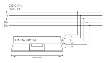
Note: Battery must be connected before mains connection.
