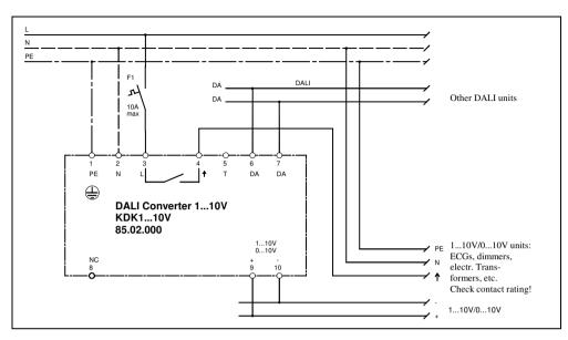
Wiring diagram: DALI Converter 1...10V in 1-button mode (Converter: 1-button switching/dimming function)
